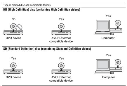
\* Install the AVCHD compatible application on your computer beforehand. Even in the case of a computer environment that satisfies system requirements, there may be noise in video playback, frames may be dropped, or sound may be lost intermittently. (This does not depend on the quality of the created disc.)
